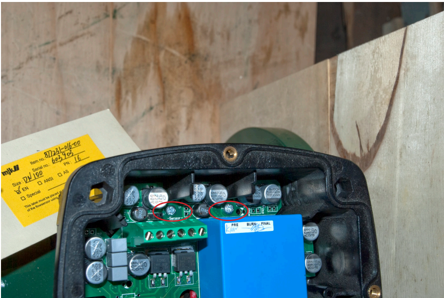
6. Mount converter pc board in the cabinet
