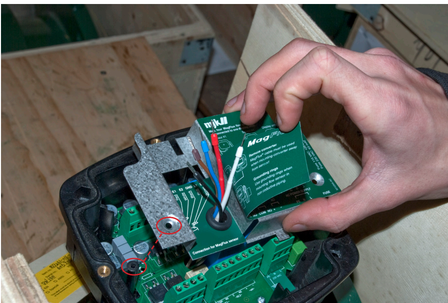
9. Fasten cover plate, using 2 screws
