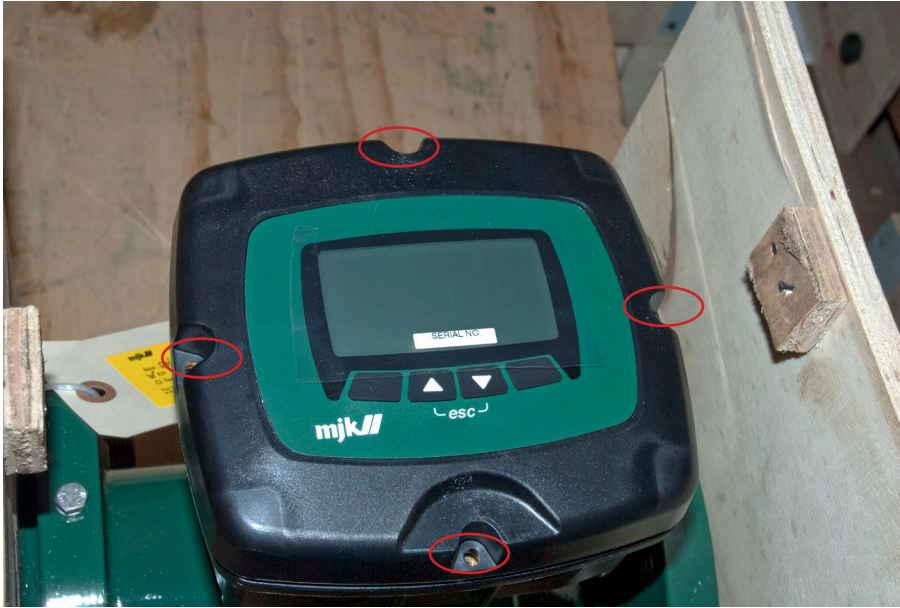
12. Fasten Display using 4 screws
